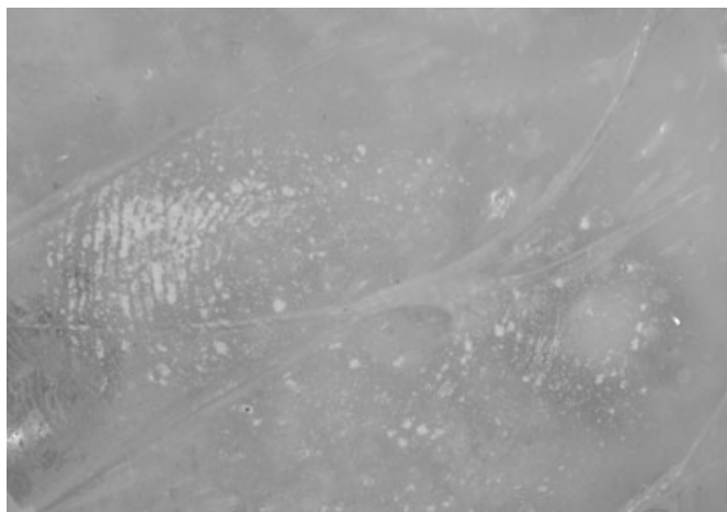
FIG. 4—Latent fingerprint partially visualized by cyanoacrylate fuming, p -dimethylaminobenzaldehyde vapor staining, and UV irradiation (365 nm); the fingerprint had been deposited on a smooth surface of polycyanoacrylate plate in advance.
